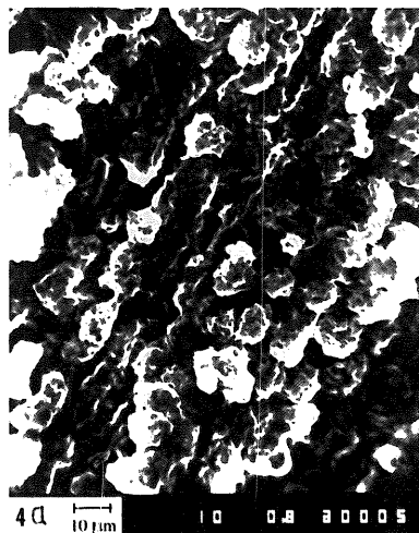
Fig. 4. Electrodeposited Li from a 1 M LiClO 4 -(PC-EC-DME) (1:1:2) solution: (a) without any additives, and (b) with 0.025 M TEAFOS as additive.
