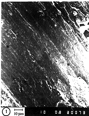
Fig. 1. Surface of the uncontaminated Li substrate before any electrochemical treatment.
